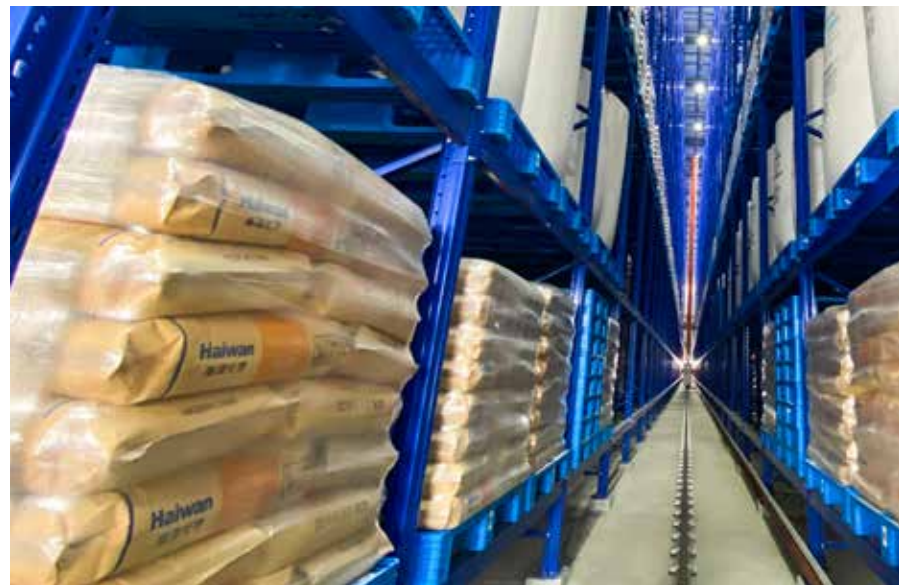
海湾化学智能化立体仓库。 Intelligent three-dimensional warehouse of Haiwan Chemical.
